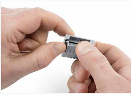
Open the Gelbox at the side latches.
