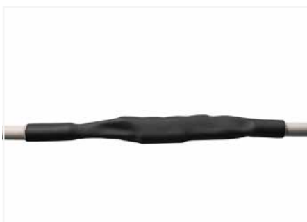
The shrinking process is only completed when the shrink tube is tightly connected to the cable and the adhesive has visibly melted (see photo).
