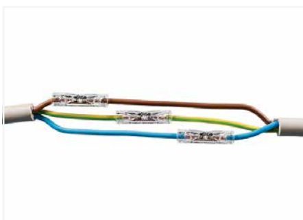
Strip 10 mm conductor per specification and insert connector (example shows staggered connectors).
