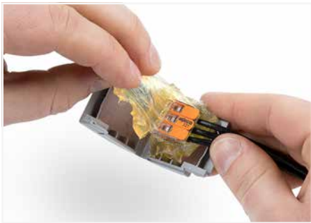
Re-accessible: Open the Gelbox, remove the gel, open the connector and rewire with new components.
