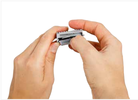
Open the Gelbox at the side latches.
