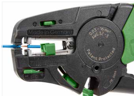
Partially stripping a conductor.
