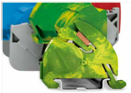
Ground busbar carrier (812-141): Offers a receptacle with locking device for (10 x 3) mm busbar. Contact between the busbar and rail is made automatically by simply snapping the carrier onto the DIN-35 rail. One end of the busbar is mounted into the ground busbar carrier, the other end is inserted into the middle position of the insulated busbar carrier.
