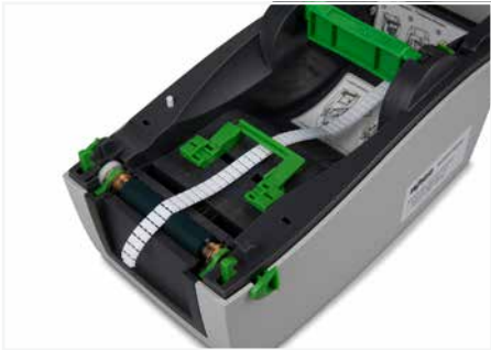
Guide the marker strip over the roller.
