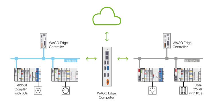
The illustration shows the interaction between various I/O devices (here: a motor, a pump, a light and hot water) acting as sensors and/or actuators and how these are integrated into the overall system (here: building automation) using WAGO Edge Controllers and WAGO Edge Computers.
