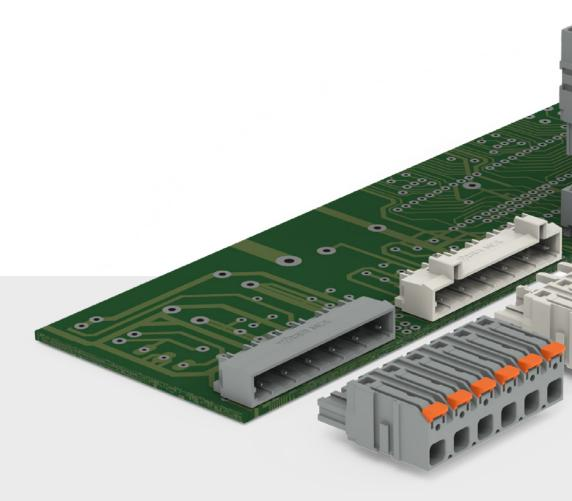
The *MCS* MIDI is suitable for conductor crosssections of up to 4 mm<sup>2</sup> with fine-stranded conductors. Conductors with ferrules or insulation can be accommodated up to 2.5 mm<sup>2</sup>. With the *MCS* MIDI featuring levers and a pin spacing of 7.5 mm, the power connection for devices across a wide performance range can now be established with uniform, tool-free handling.
