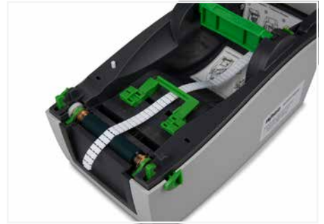
Guide the marker strip over the roller.
