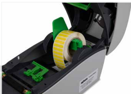
Loosen the center bar, loosen the wing and place material on the bar.
